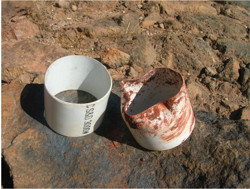
Figure 2.9: Plastic collars before (left) and after (right) inserting into the ground in Passo del Vento.
