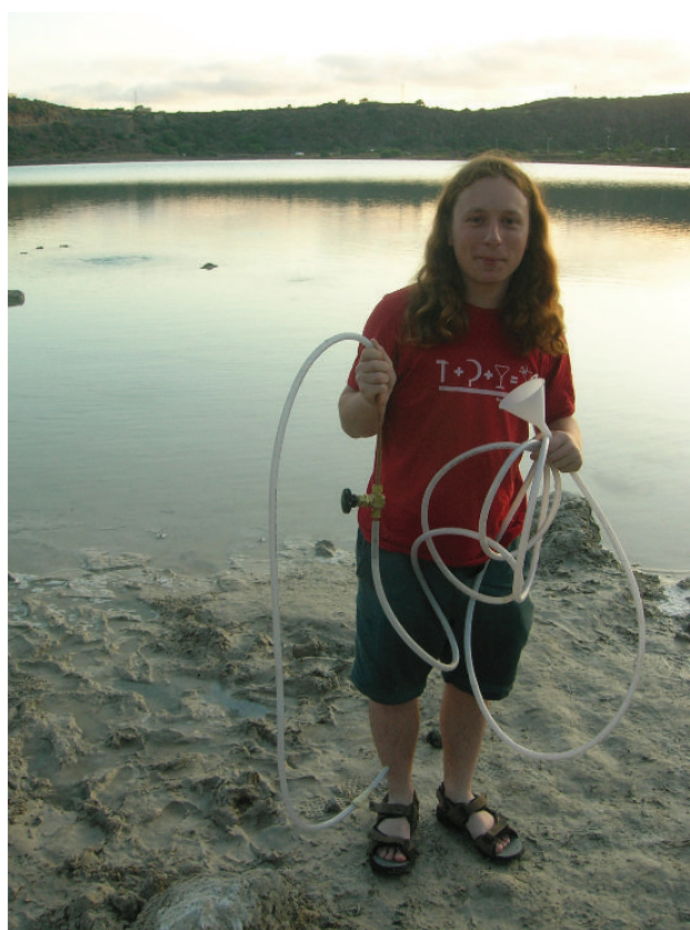
Figure 2.10: Apparatus used to collect gas samples from Specchio de Venere. In the background, to the left, is a bubbling source where gas was collected.
